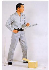
The line-throwing device can be used from ship to ship or ship to sea shore and also is siutable for rescue operation at sea and on land.
